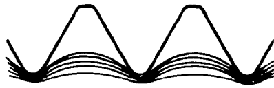
FLOW LINES, ROLLED THREAD FIGURE 3
