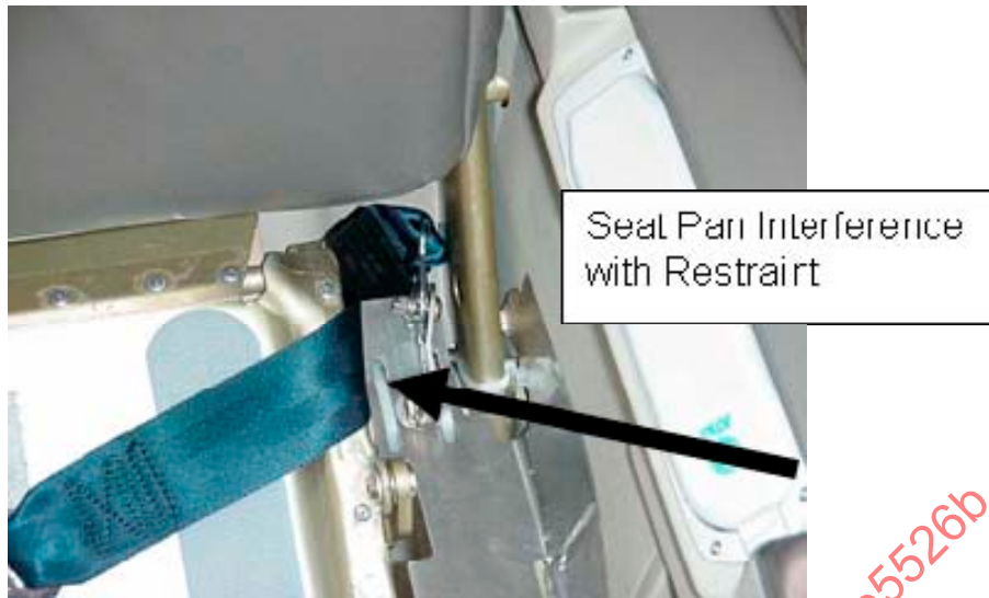
FIGURE 3.2C - AN EXAMPLE OF A DESIGN TO AVOID
