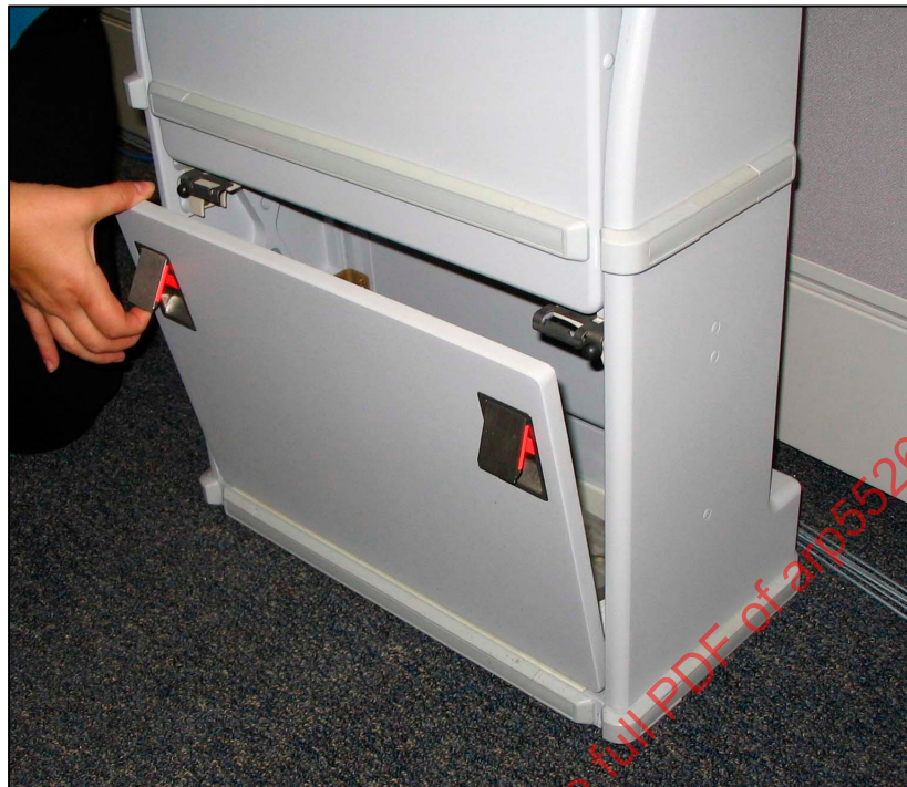
FIGURE 10 - THIS IS A SPRING MOUNTED STOWAGE BOX DOOR. IT IS AN EXAMPLE OF A TYPE 4A SCORE FROM THE INJURY POTENTIAL ANALYSIS TABLE BASED ON SPRING FORCE POTENTIAL.
