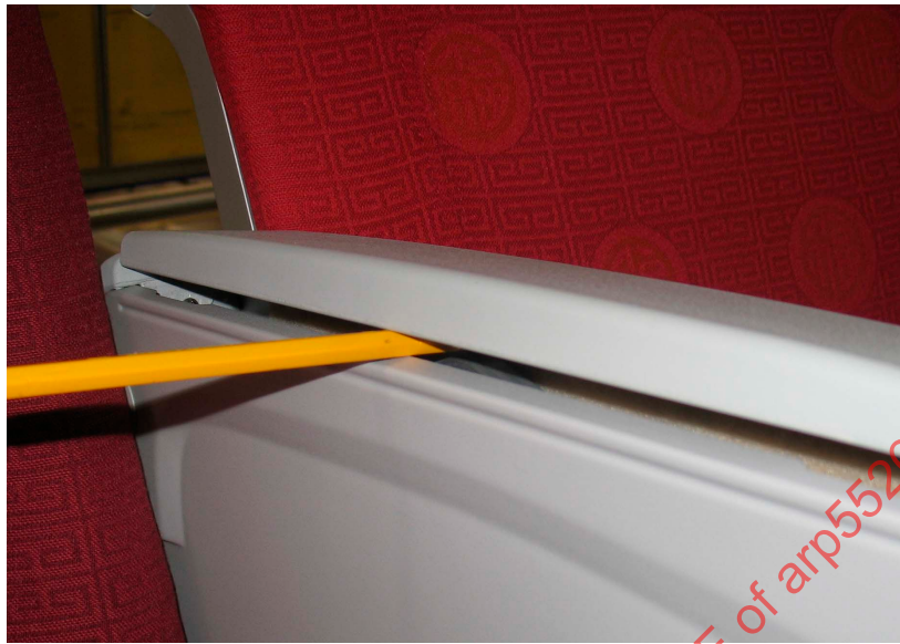
FIGURE 8 - THIS IS THE ARM CAP FOR AN IN-ARM TRAY TABLE SEAT. IT IS AN EXAMPLE OF A TYPE 1A SCORE FROM THE INJURY POTENTIAL ANALYSIS TABLE.
