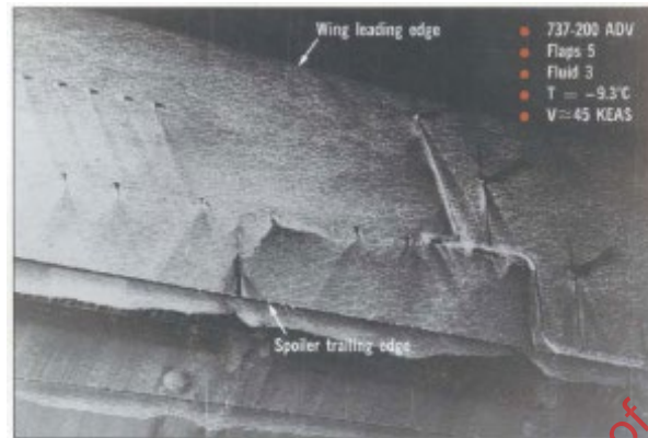
Figure A2 - Ultraviolet fluorescent photograph of a fluid 8 seconds after brake release
