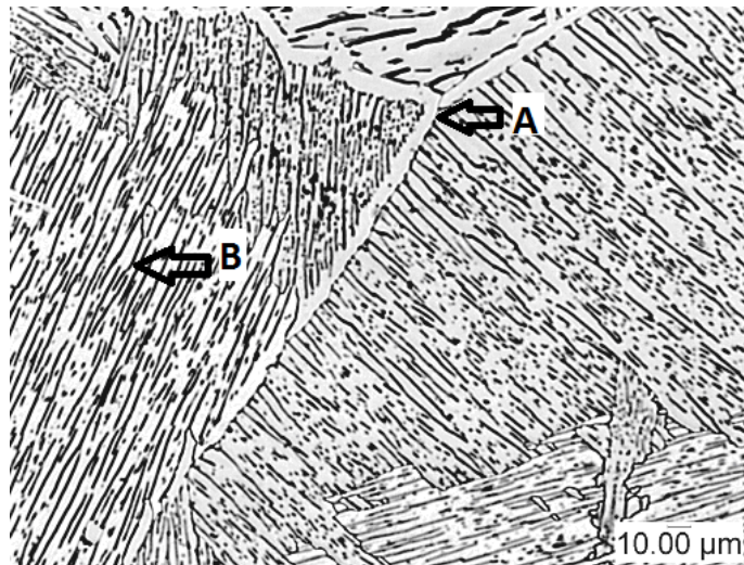
ETCHANT: KROLL'S 300X ALLOY 6Al-4V. ACICULAR ALPHA COLONIES IN PRIOR BETA GRAINS. "A" = GRAIN BOUNDARY ALPHA, "B" = ACICULAR ALPHA COLONIES.
