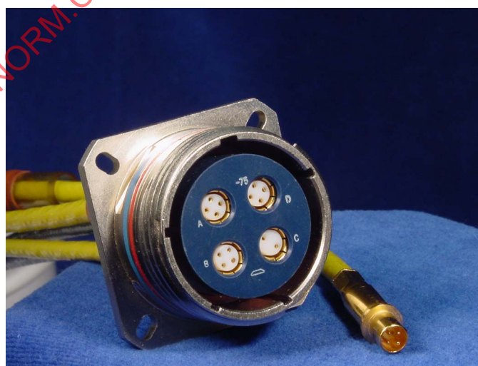
FIGURE 7 - Example of MIL-DTL-38999 Connector Inserts that Support Quadrax Inserts
