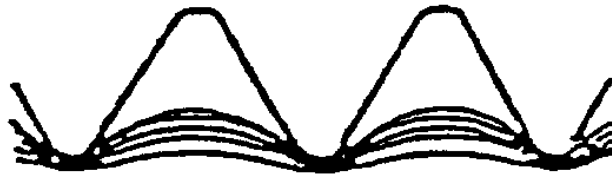
FIGURE 3 - FLOW LINES, ROLLED THREAD
