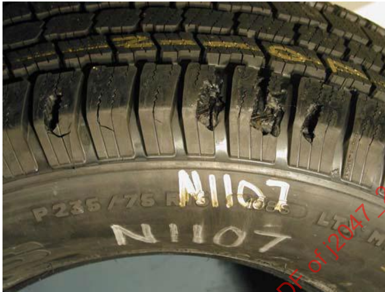
FIGURE 31 – AN EXAMPLE OF TREAD CHUNKING
