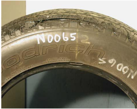
FIGURE 29 – BELT EDGE SEPARATION EXAMPLES
