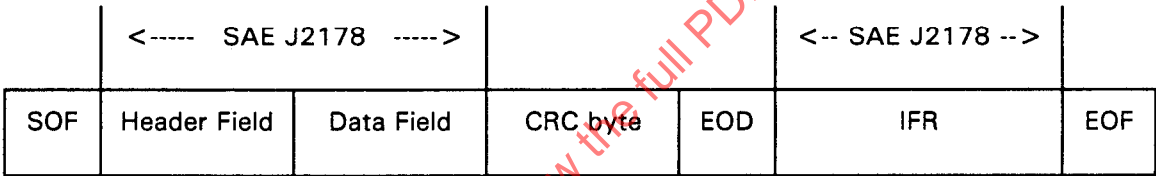
FIGURE 2—SCOPE OF SAE J2178 FOR A SAE J1850 FRAME WITH IN-FRAME RESPONSE (IFR)
