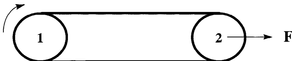
Figure 3 - Belt pilling test stand configuration
