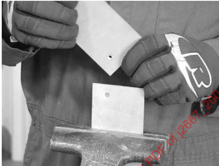
FIGURE 5—THE TWIST TEST CREATES A TEAROUT HOLE IN ONE COUPON AND A NUGGET ON THE OTHER
