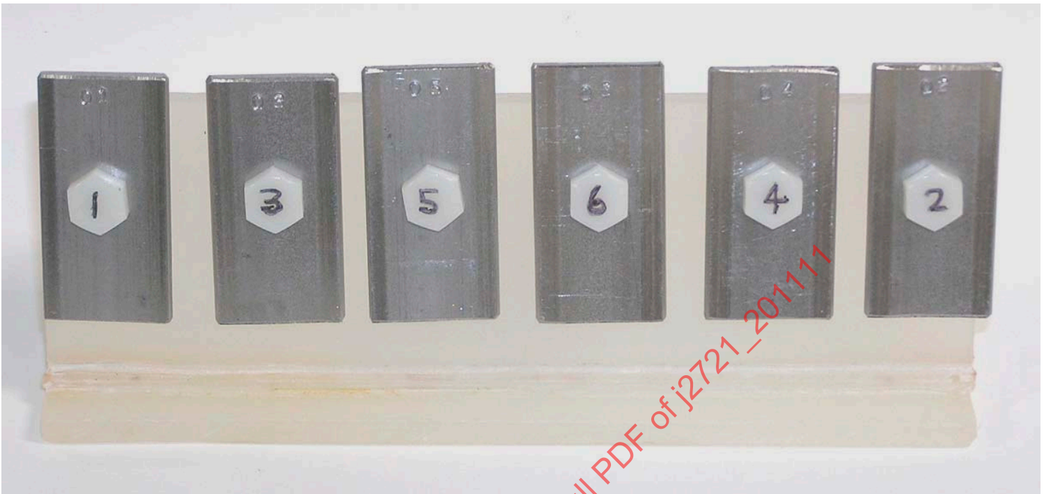
FIGURE 2A - CORROSION MASS LOSS COUPONS MOUNTED IN RACK – FRONT VIEW
