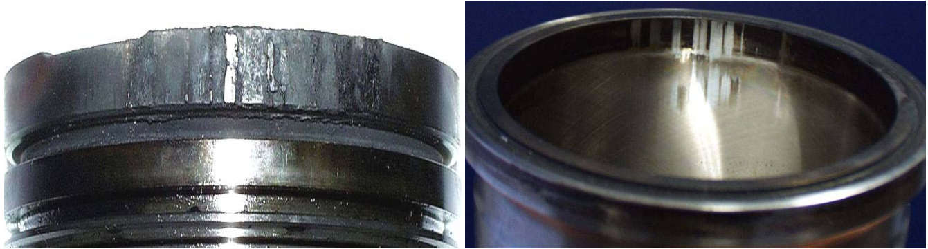
FIGURE 5 - EXAMPLE OF CARBON POLISHING
