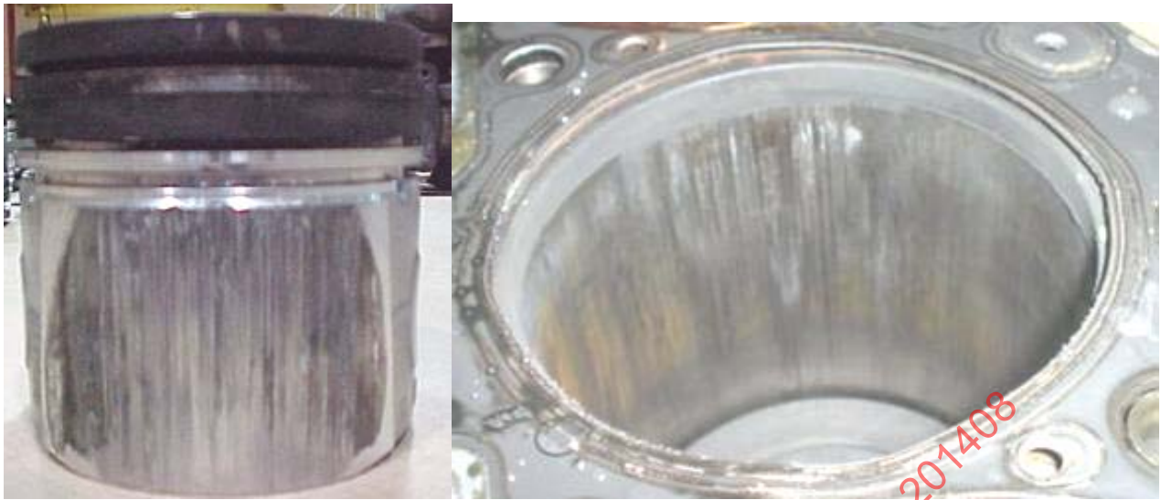
FIGURE 4 - EXAMPLE OF PISTON SCUFF
