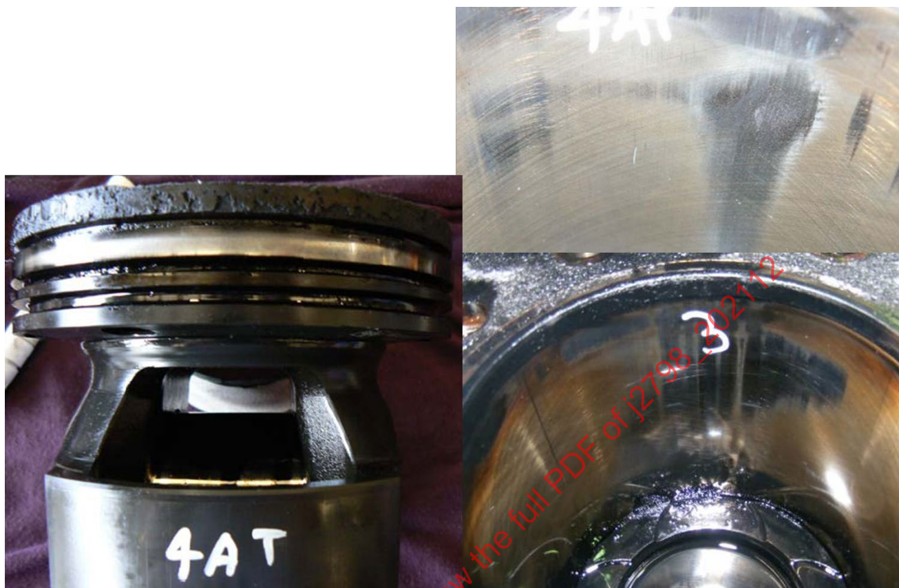
Figure 5 - Example of carbon polishing
