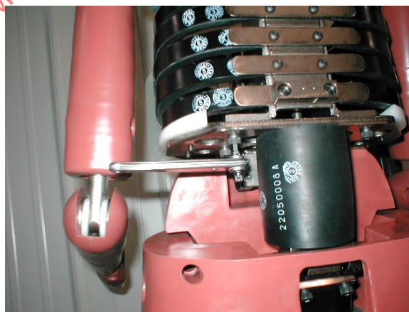
Figure 12 - Removing upper torso from lower torso
