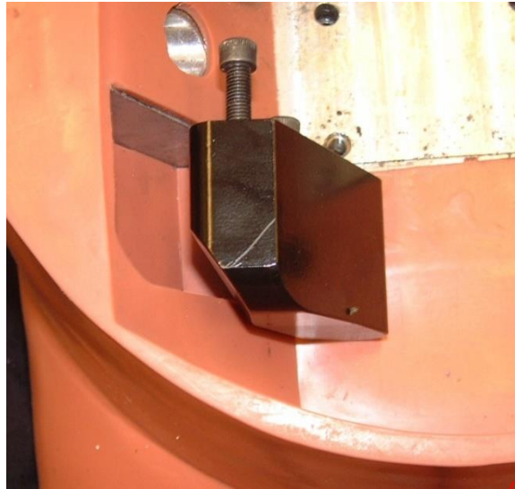
Figure 27 - Orientation of right iliac load cell
