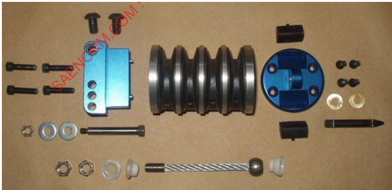
Figure 10 - Components of neck assembly
