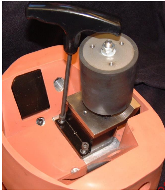
Figure 22 - Remove lumbar spine from pelvis using two SHCS accessible from the top
