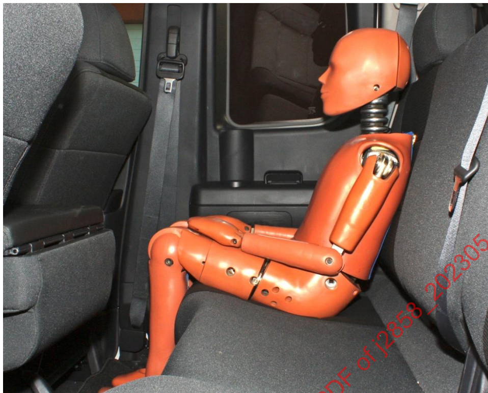
Figure 4 - Side view of Hybrid III 10YO in slouched posture
