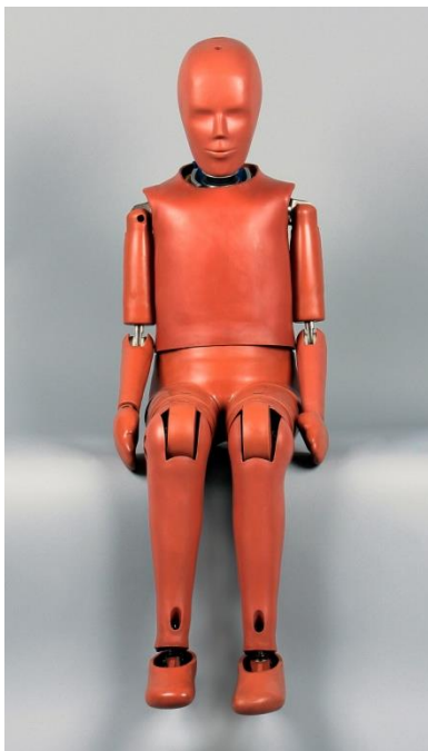
Figure 2 - Front view of Hybrid III 10YO
