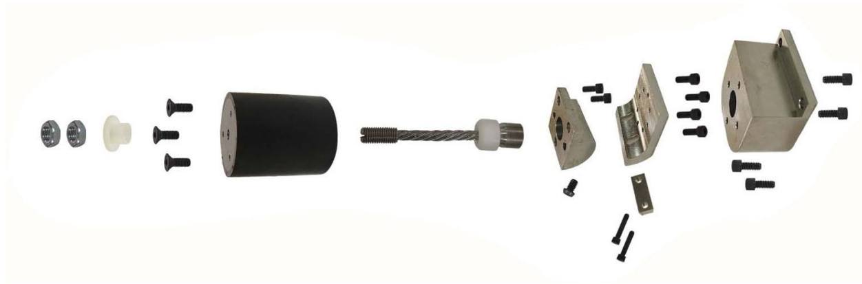
Figure 24 - Exploded view of lumbar spine assembly
