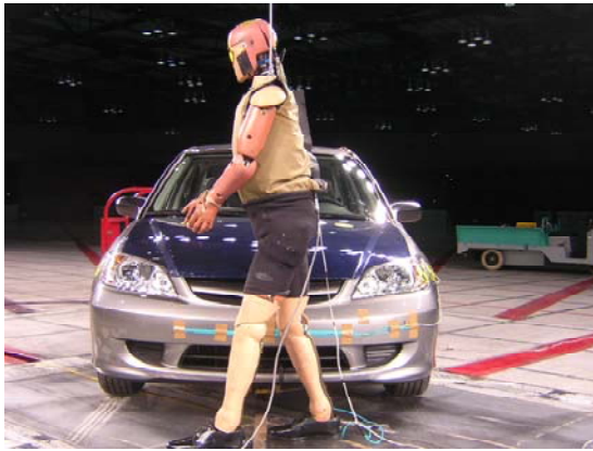
FIGURE D1 - TEST CONFIGURATION FOR POLAR II DURABILITY TESTING
