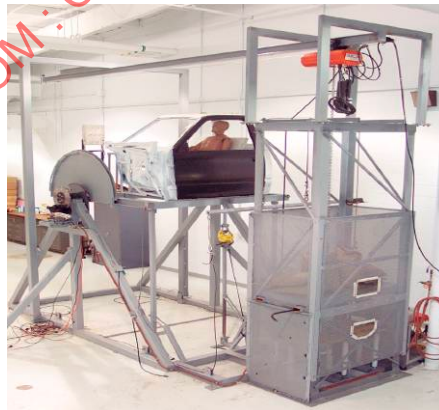
FIGURE 25 - DYNAMIC ROLLOVER FIXTURE (DRF)
