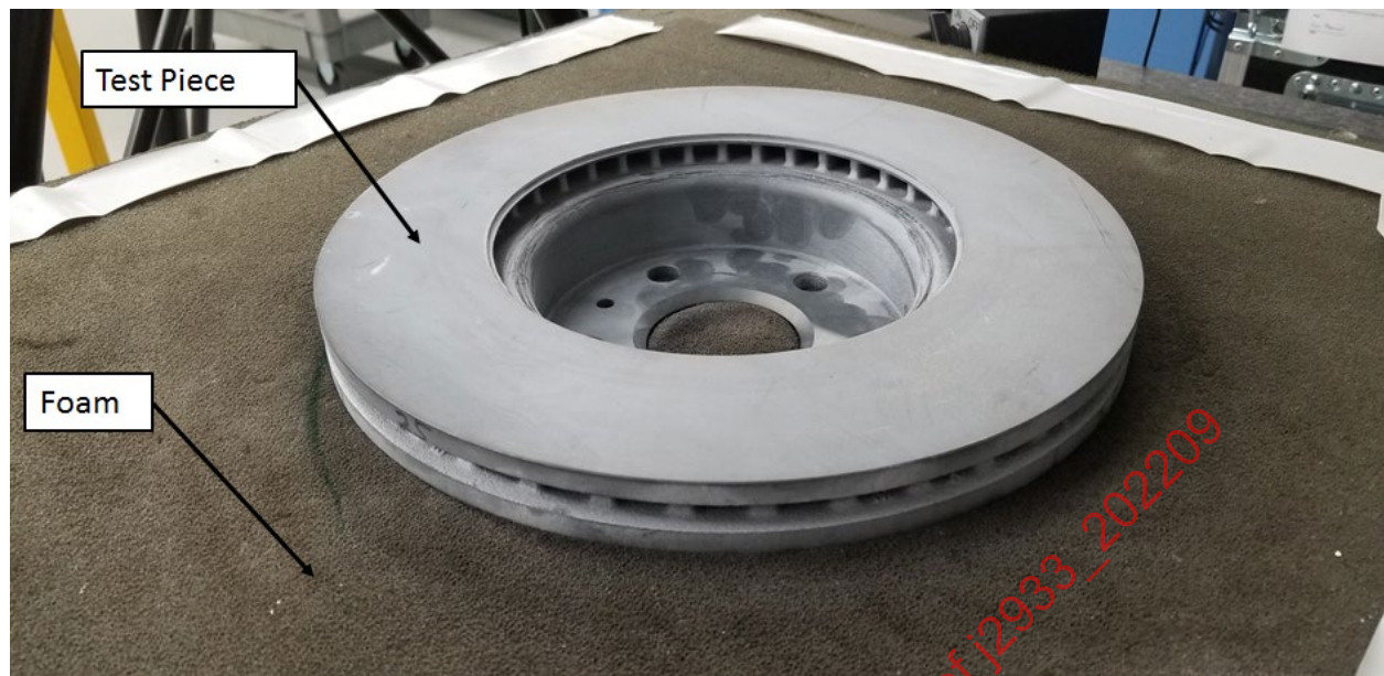
Figure A1 - Foam used to support brake components in free-free condition
