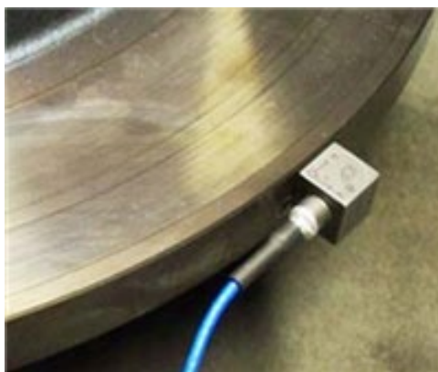
Figure 2 - Impact and accelerometer configuration
