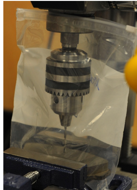
Figure 3 - A schematic representation of a disc pad and lining showing the area that can be used for sample collection (gray shaded). Also shown (right) is a brake friction assembly in a sealable plastic bag ready for the start of sample collection
