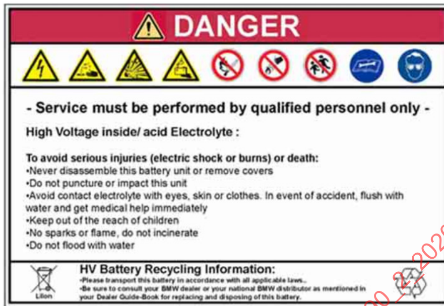
Figure 5 - Example multi hazard battery label
