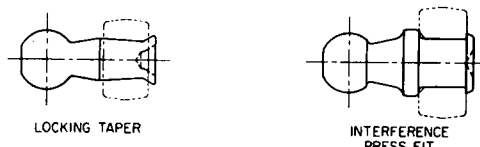
FIG. 3 - PERMANENTLY ATTACHED STUDS--RIVETED, WELDED, SPUN, OR STAKED
