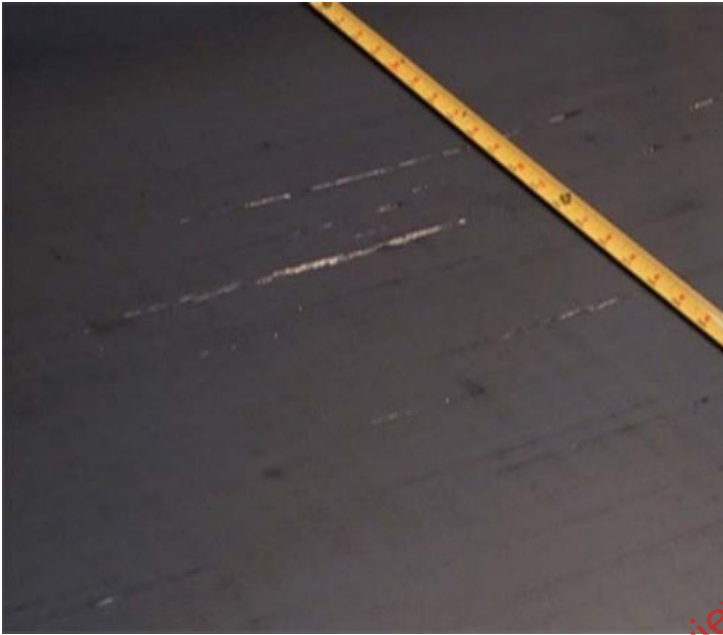
Galvanized scratches (left); Galvanized scratches under 50X magnification (right)
