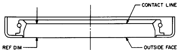
FIG. 11—CONTACT LINE HEIGHT VARIATION
