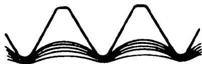
FLOW LINES, ROLLED THREAD FIGURE 3
