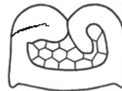
FIGURE 4.3.5-1 - CONDUCTOR CRIMP CROSS-SECTION CRITERIA
