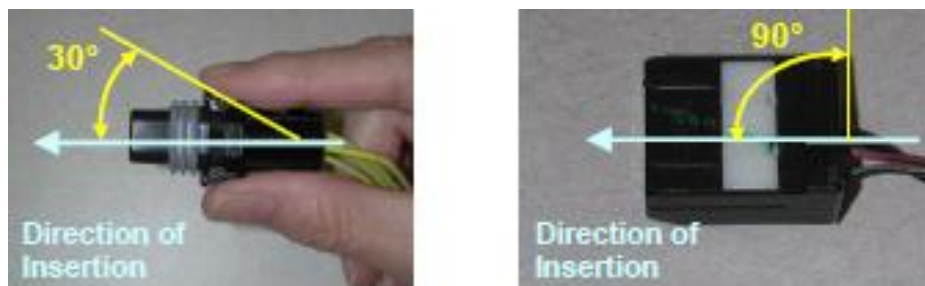
Figure 2: Contact Surface Angle. Acceptable Contact Surface: Optimally angled between 30° and 90° from the direction of the force insertion.
