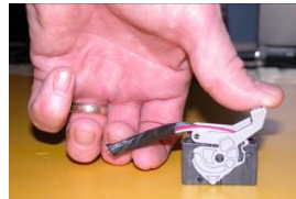
Figure 8: Unconstrained Lever Lock Connector example: Fingers / thumbs are not confined to the space between the lever arms.
