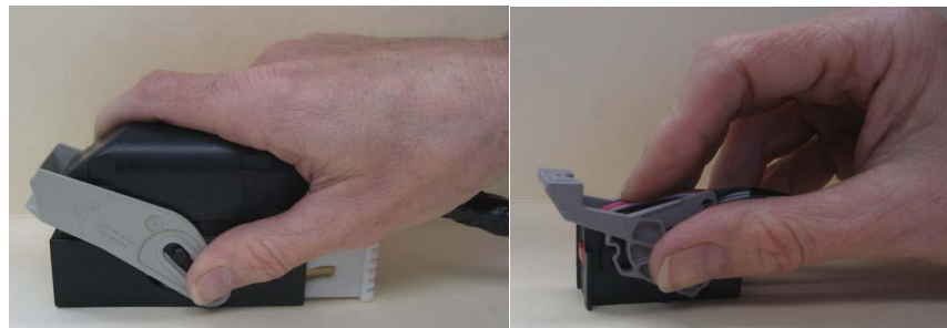
Figure 15: Typical Postures used to position mechanical assist connectors
